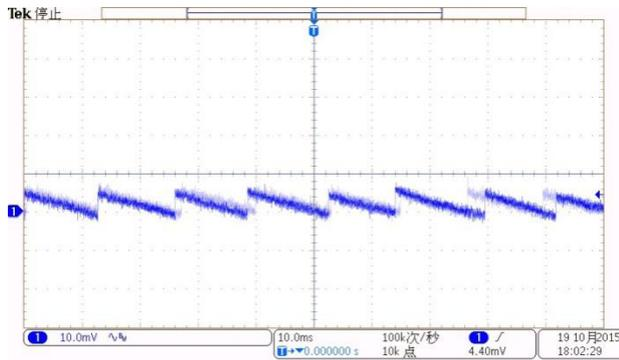
(13) Output Ripple for IOU=200mA
