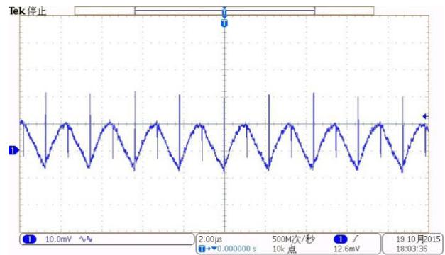
(14) SW waveform for No Load
