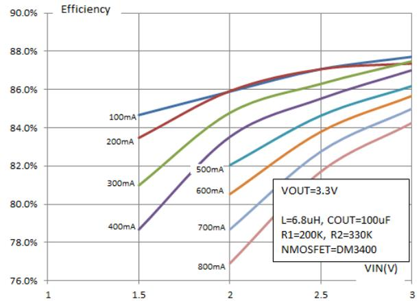
(8) Load Regulation for Expanded Current
