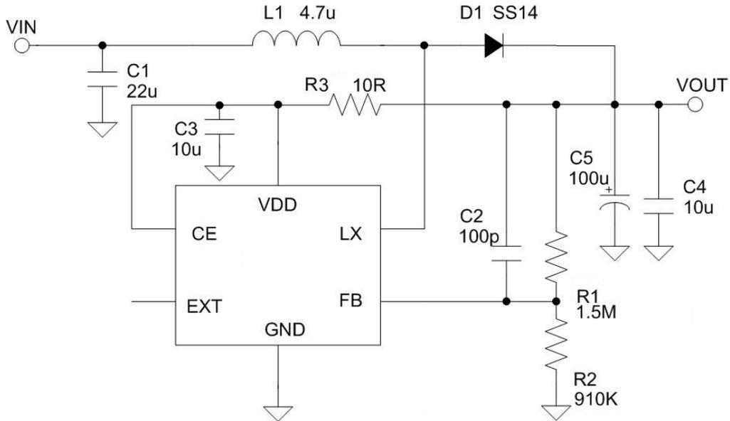
The basic application circuit for UCT1301 is shown as above figure. The output voltage VOUT can be derived from:
