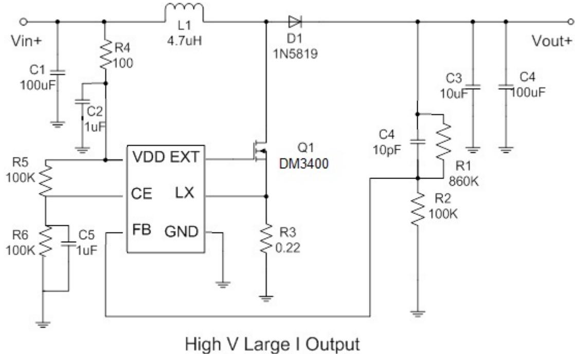
Adding an external power MOSFET DM3400 (or NPN) still driven by the EXT pin of the UCT1301 as the above figure can get VOUT higher than 5V. The VOUT of the above circuit is:
