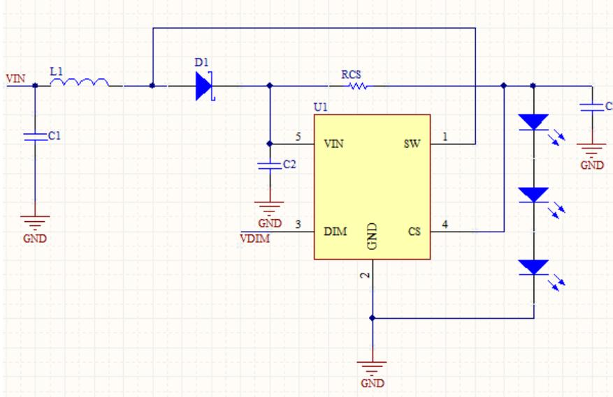
In this case the VIN Voltage is lower than the total LED string Voltage. The minimum VIN Voltage is 4V.
