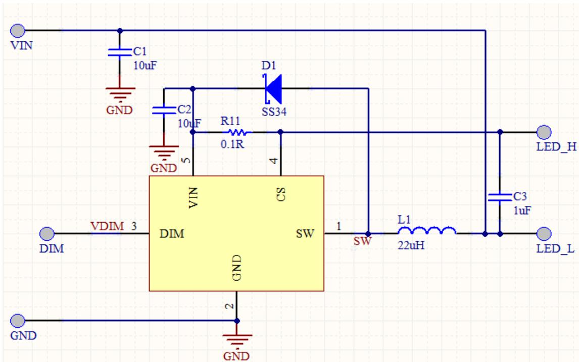
With this circuit the VIN Voltage can be either higher or lower than the LED string Voltage. Note that the Maximum VIN+VLED shall be lower than the device OVP voltage, which is 40V typically.
