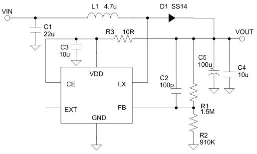
The basic application circuit for UCT1301 is shown as above figure. The output voltage VOUT can be derived from:
