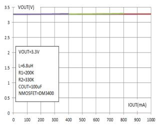
(10) Start-up Voltage vs IOUT for Expanded Current
