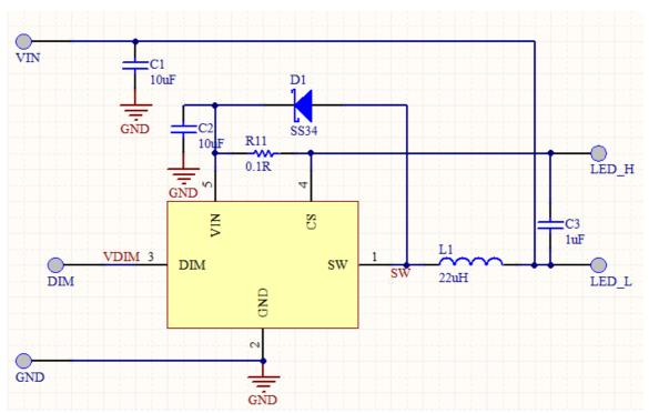
With this circuit the VIN Voltage can be either higher or lower than the LED string Voltage. Note that the Maximum VIN+VLED shall be lower than the device OVP voltage, which is 44V typically.
