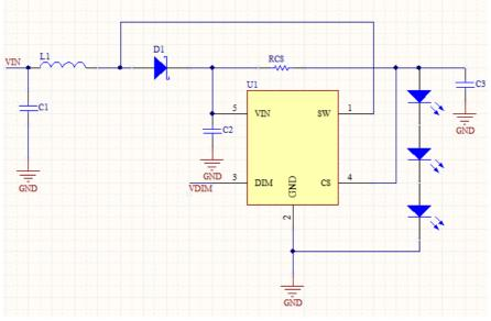
In this case the VIN Voltage is lower than the total LED string Voltage. The minimum VIN Voltage is 3.5V.
