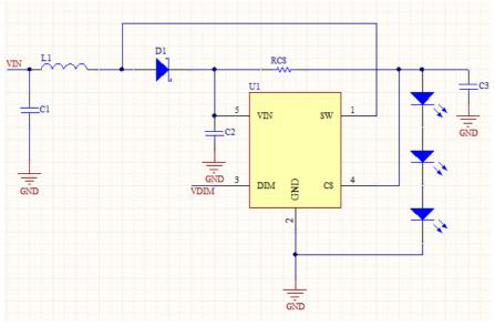
In this case the VIN Voltage is lower than the total LED string Voltage. The minimum VIN Voltage is 4V.
