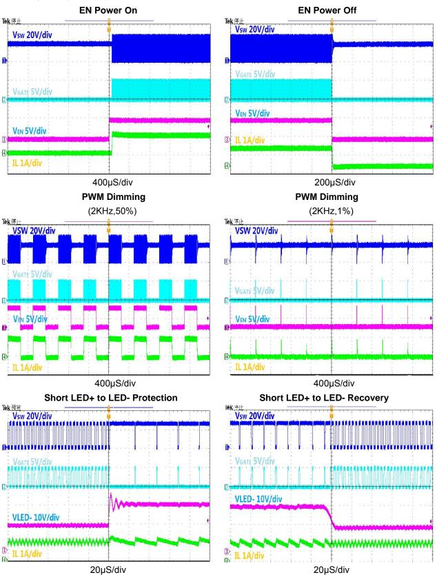
$V_{IN}$ =24V,3LEDs, $I_{OUT}$ =1A, $T_{A}$ =25 $^{\circ}$ C, unless otherwise noted.
